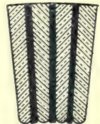
FIG. 134.—Sketch showing rounded edges of Commutator Segments.
